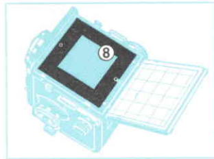
Inserting the Screen Mask (removing the focusing hood)
